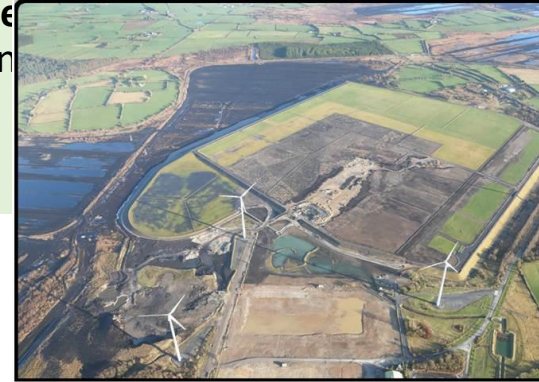
2018: Lisheen Tailings Management Facility - remediation almost complete. The cover material in the 2015 photograph have been used and the area re-vegetated. Note also removal of infrastructure (bottom centre). Photo credit: Vedanta zinc international
